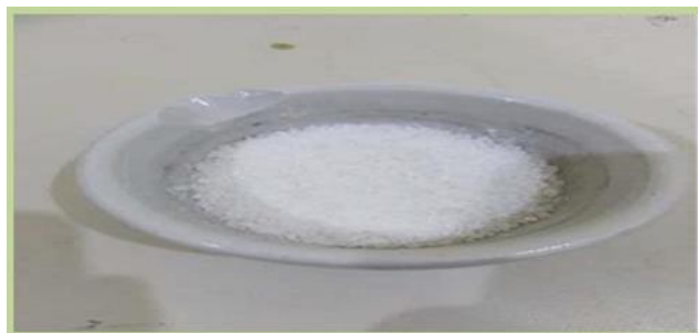
Fig. (3): Prepared gamma alumina after drying.
