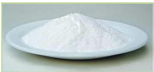
Fig. (4): Final prepared Nano \gamma -alumina
