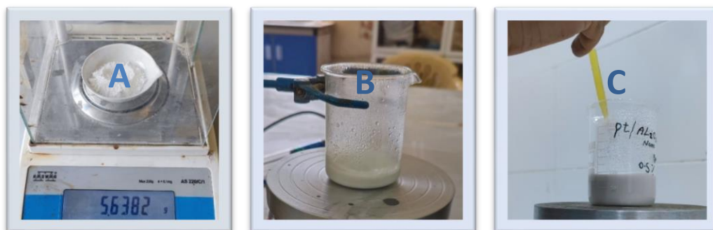
Fig. (2): (A) Weighing \gamma\text{-Al}_2\text{O}_3 nanocatalyst (B) \gamma\text{-Al}_2\text{O}_3 particles dissolution with distilled water (C) Loading with Pt-metal
