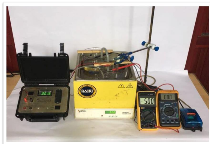
Fig. (2): Displays the equipment utilized to investigate free and galvanic corrosion.
