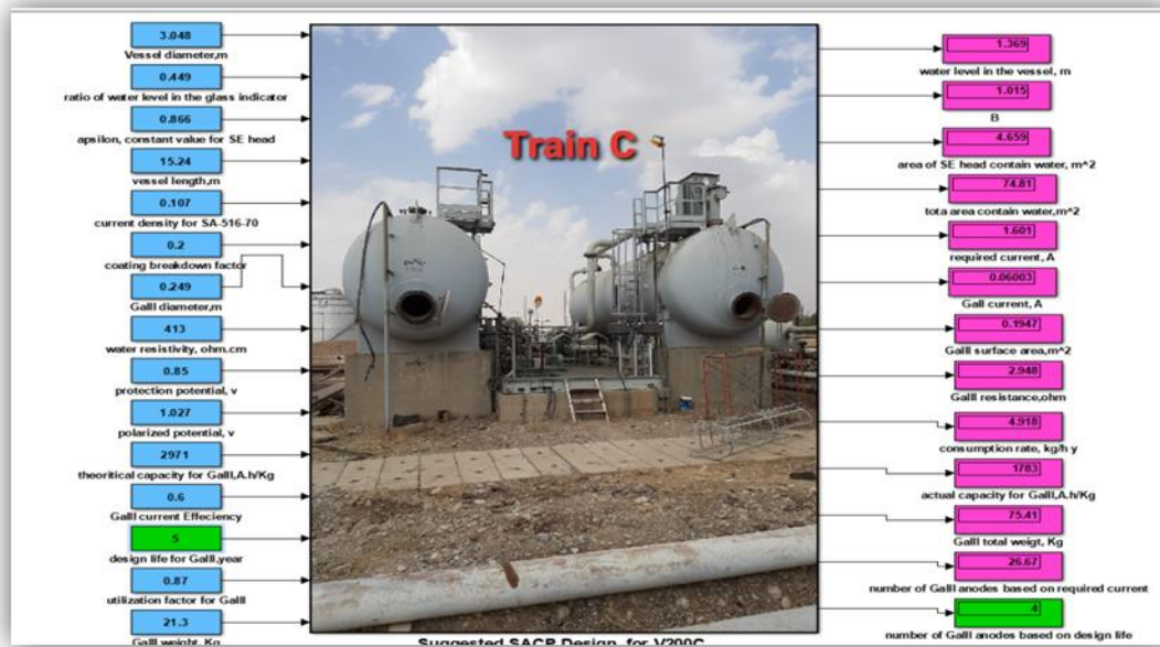
Fig. (9): Matlab simulation of new SACP design for dehydrator
