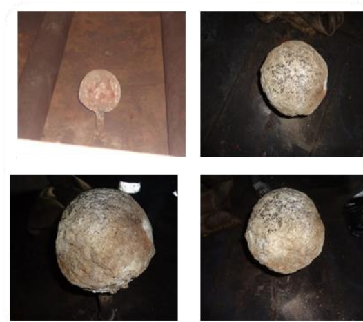
Fig. (1): Consumable and deposited GaIII anodes
