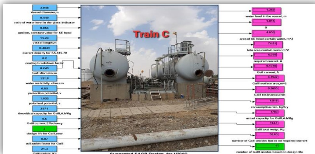
Fig. (10): Matlab simulation of new SACP design for desalter
