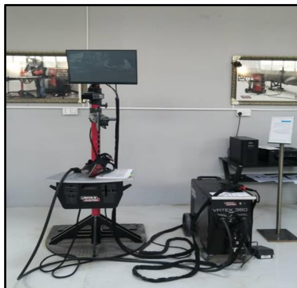
Fig. (2): The virtual welding system setup
