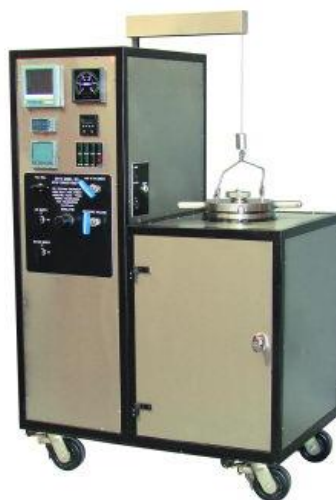
Fig. (5): HPHT Consistometer Apparatus
